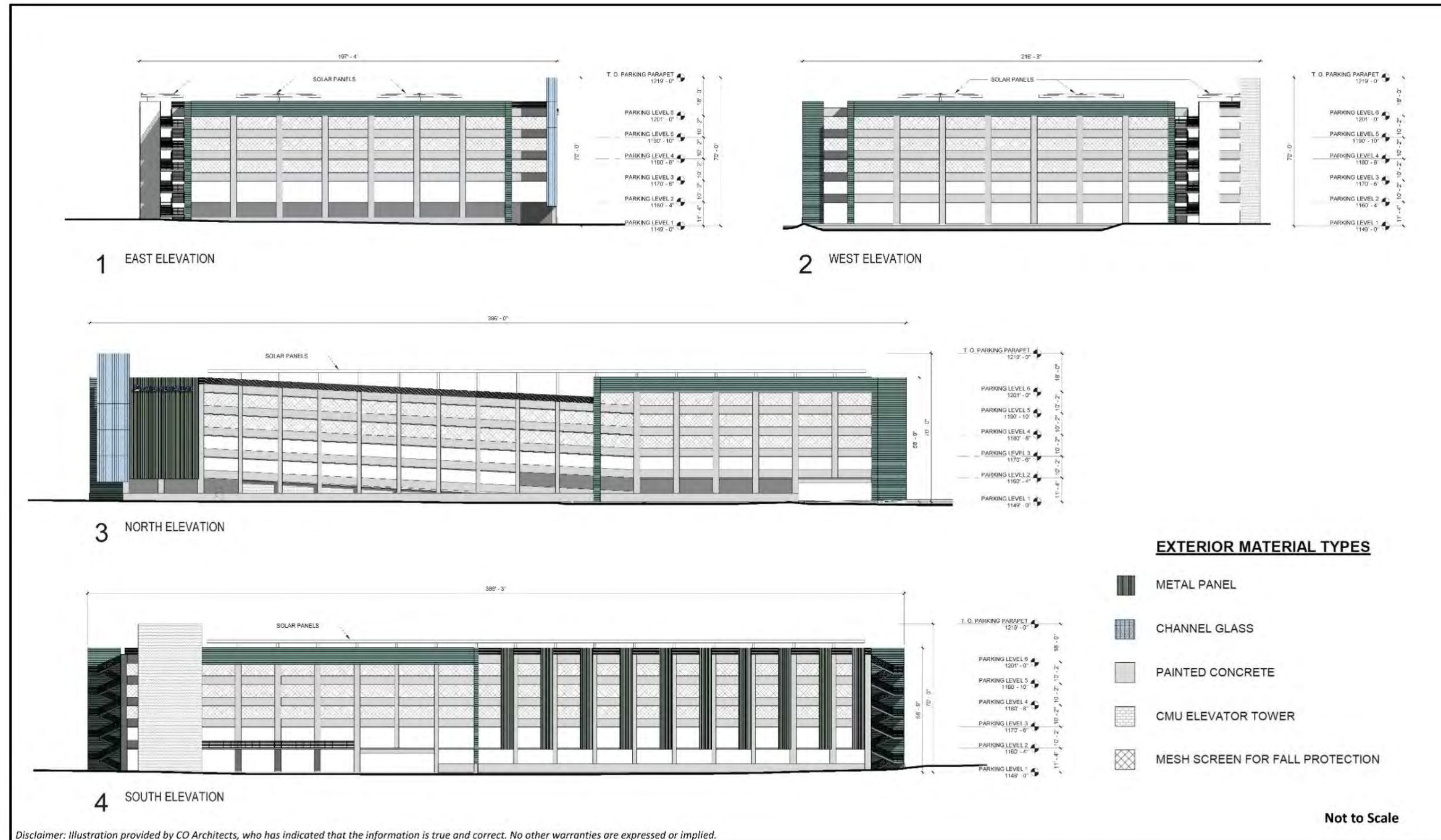
Figure 3.3-13 PARKING STRUCTURE ELEVATIONS
