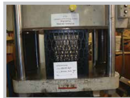
Unconfined Compression Test
